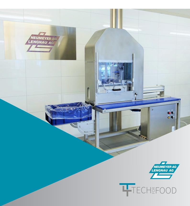
The meat press press it has been developped to press unshaply beef cuts (pork, beef, veal or poultry) into a even shape. The yield and weight accuracy during the subsequent portioning and slicing process is getting considerably improved. The intended raw material has to be slightly frosted or consistent defrosted at -2 to -3°C (product specific).
