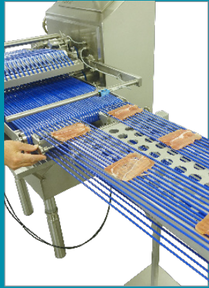
Hand over ridge & adjustable track control
